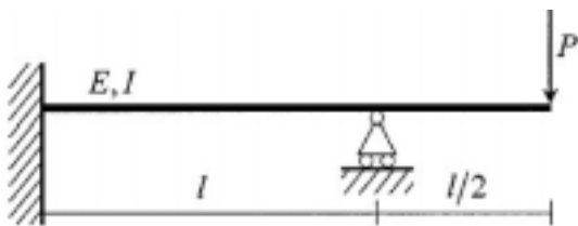
Fig. 4 Statically indeterminate beam
