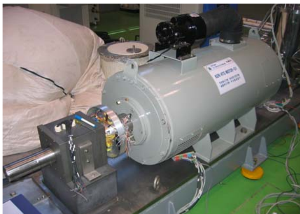
Fig. 4 Wireless transmitter attached on the shaft of superconducting motor
