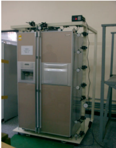
Fig.9 Flatness test configuration
