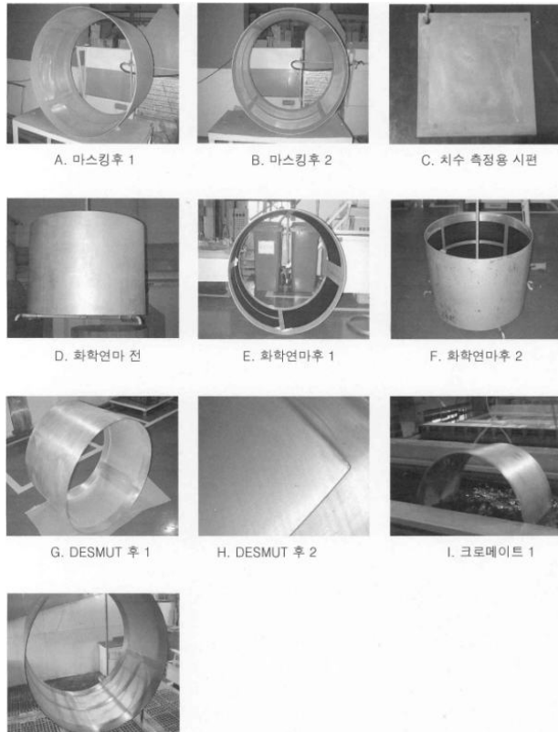
Fig. 4 Chemical milling process of cylinder
