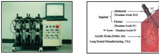
(a) In-house built smart impact tester (b) Specimen Fig. 5 Tester and specimen used in this study
