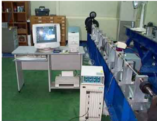
Fig. 1 Split Hopkinson Pressure Bars system
