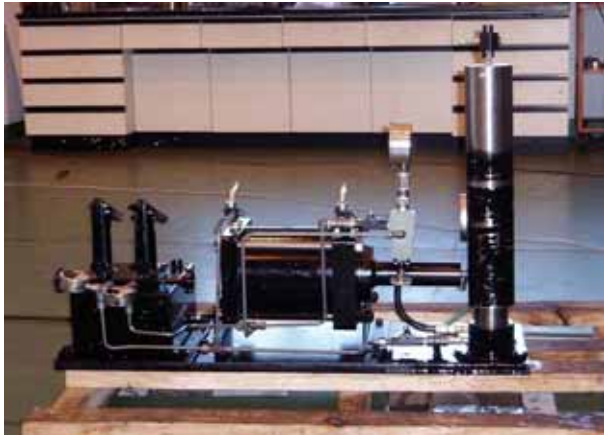
Fig. 3 Burst pressure test equipment
