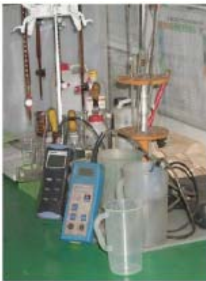
Photo. 1 Measuring apparatus for corrosion potential measure
