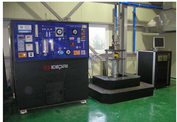
Fig. 5 Photograph of low-cycle fatigue test rig
