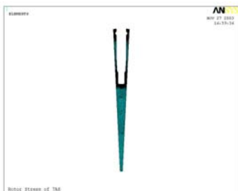
Fig. 8 FEM Model of Rotor Tooth
