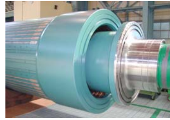
Fig. 9 Geometry of Rotor and Retaining Ring
