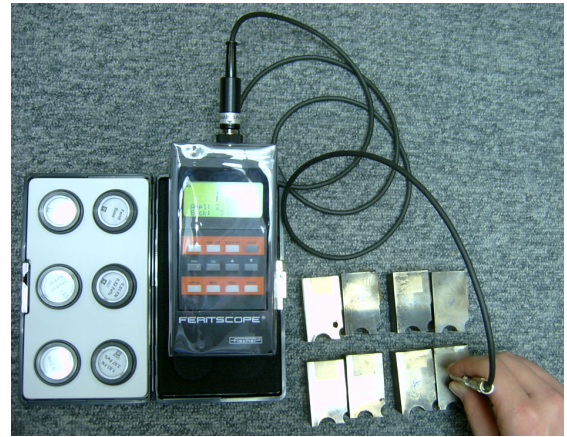
Fig. 1 Measurement of ferrite content for CT specimen using FERITSCOPE MP30
