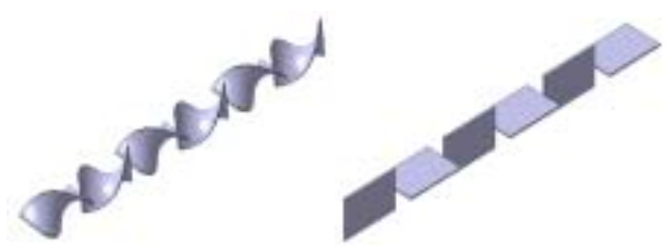
Fig. 1 Schematic diagram of Kenics and PPM elements
