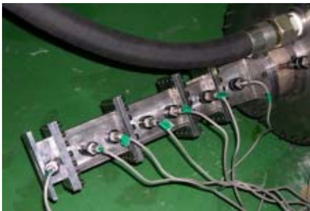
Fig. 6 Assembling supersonic diffuser
