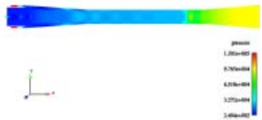
Fig. 3 Pressure contour of ejector
