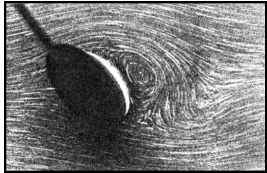
Fig. 4 Comparison of instantaneous stream line for Re = 200, \phi = 54^\circ at T^* = 2.1 : present study(top), Honji (5) (bottom).
