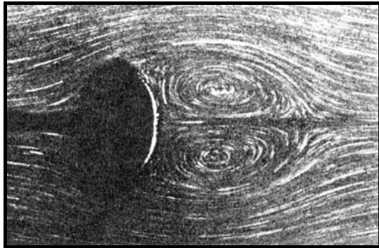
Fig. 2 Comparison of instantaneous stream line for Re = 200, \phi = 90^\circ at T^* = 4.19 : present study(top), Honji (5) (bottom).
