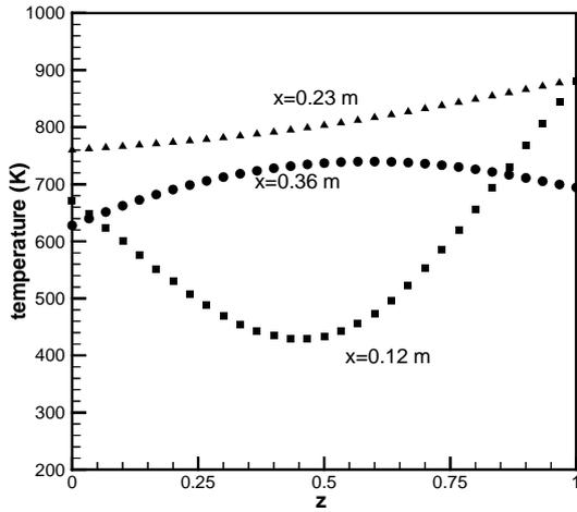
**Fig. 4** Temperature profiles at upstream, middle and downstream part along the height direction of the reactor.
