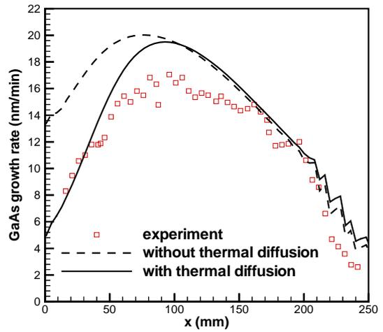
Fig. 3 Predicted growth rate curves with measured values for the GaAs film.
