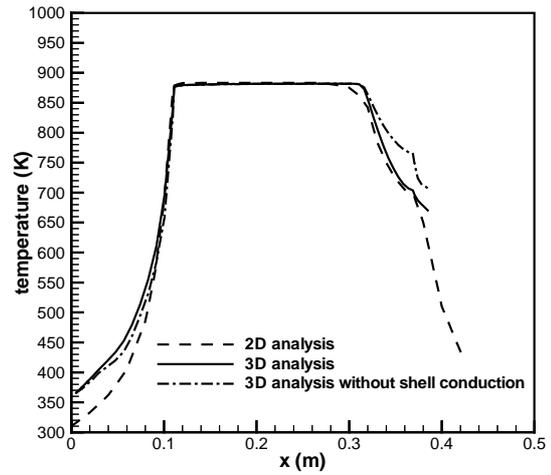
**Fig. 5** Temperature profiles of the reactor inner liner bottom wall, conduction means axial conduction within the reactor quartz walls.
