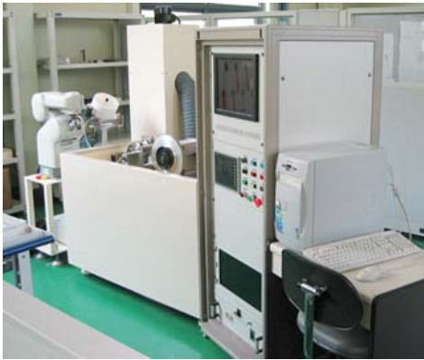
Fig. 5 Test equipment for developed coaxial grinding system
