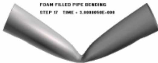
Fig. 8 Deformation pattern of the hollow cylindrical Tube
