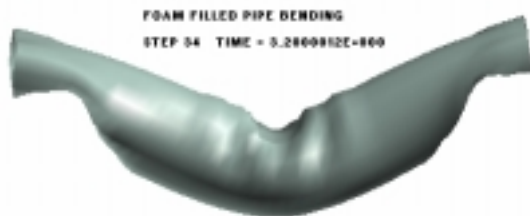
Fig. 9 Deformation pattern of 1 PC foam filled cylindrical Tube
