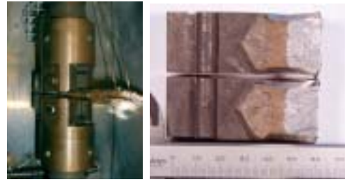
Fig. 4 J-R test specimen of CF-8A
