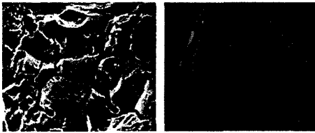
(a) Intergranular stress corrosion cracking in fracture surface (b) Secondary crack
