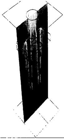
Fig. 6. Temperature distribution of heatsink (environment temperature : 25°C, without fan)
