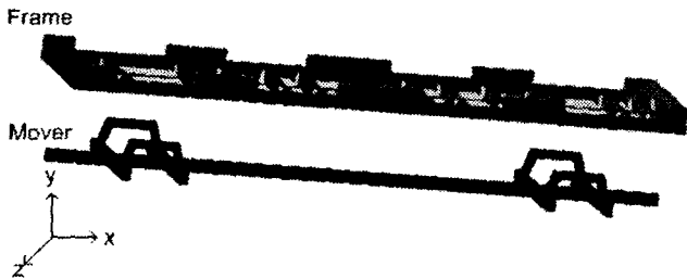
Fig. 1 Structure of shuttle car
