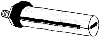
Fig 5. Handle for the force measurement (assembled)
