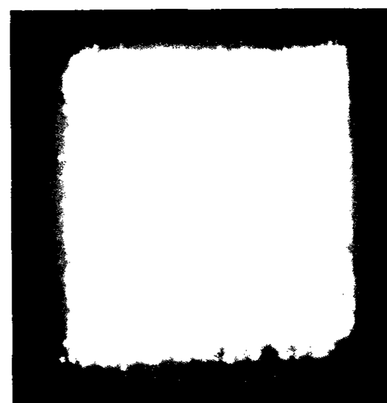
Fig. 4. Light emission pattern of the diode type CNT FED at the applied voltage, V_{a-c} of 2.0kV.
