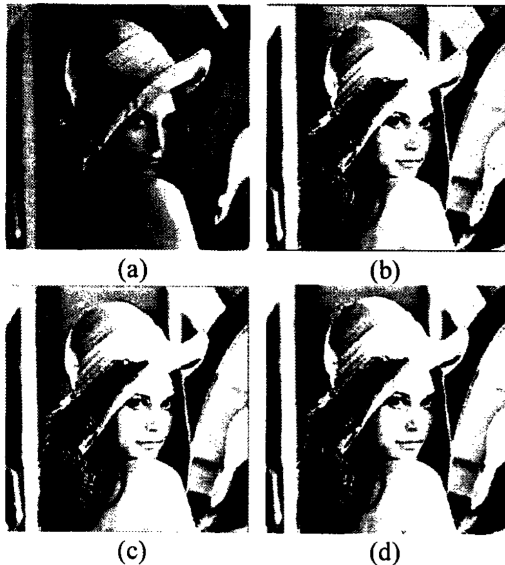
Figure 6. Simulation results on lena image: (a) original, (b) conventional method, (c) proposed method using linear approximation, and (d) proposed image enhancement methods
