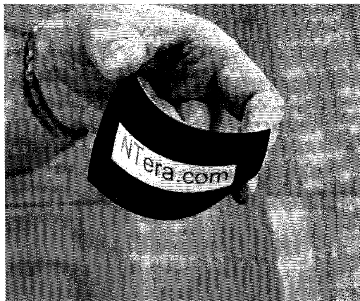
Figure 4 Flexible static display device operating under flexing and "Memory" condition
