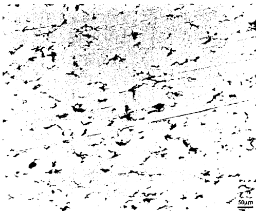
Fig.3 The optical image of GNF-Al composites
