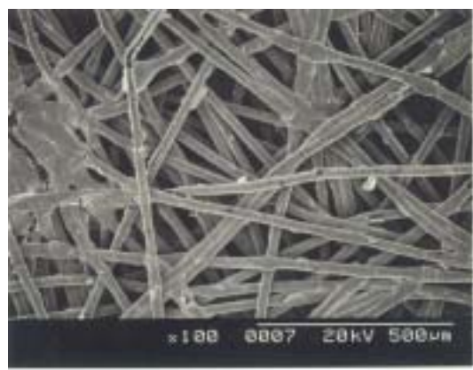
Fig 3. SEM of Nickel and Copper metal plating layer on Non-Woven PET samples (SB-50).
