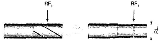
Fig. 1 Schematic diagram for determination of a reference cutting force to avoid breakage of tool shank[8].
