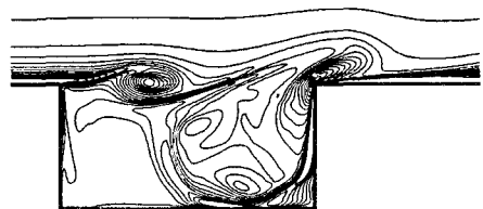
(a) Vorticity contours at an instant (20 levels between non-dimensional vorticity, \omega D/U_\infty = -7 and 3)
