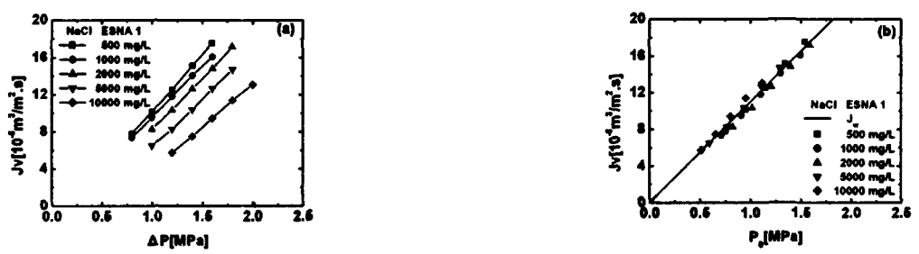
Fig. 1 The permeate volume flux of ESNA 1 membrane to NaCl as functions of the applied pressure (a) and the effective pressure (b) at different feed concentrations.
