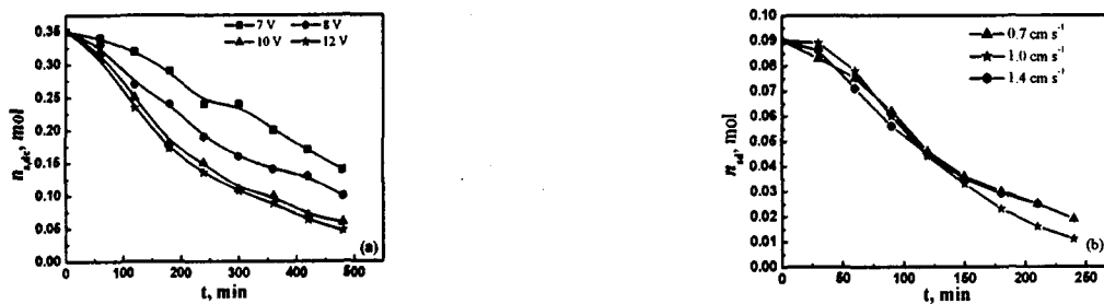
Fig.3 Molar number of organic acids salts in dilute compartment vs. operation time under different potentials (a) and flow rate (b) (a: u=1.03 \text{ cm s}^{-1} , V_{dc}=3 \text{ L} ; b: U=7 \text{ V} , V_{dc}=1 \text{ L} )
