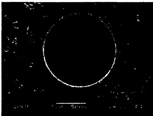
(a) Entrance of machined hole ( \phi 122 \mu\text{m} )
