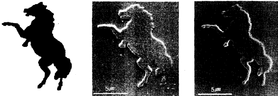
Fig.1 (a) Bitmap image of a horse. (b) SEM image of replicated horse figure without COA, and (c) with COA.
