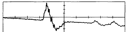
Fig. 6. typical signal of volumetric flaw
