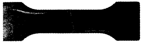
(a) Specimen of weld-line position is middle
