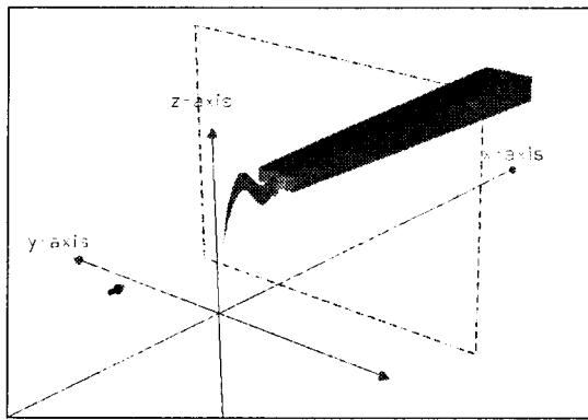
Fig. 10 3-dimensional plume behavior with CORMIX2
