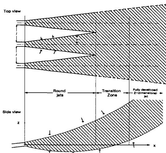
Fig. 2 Jets merging from the unidirectional diffuser
