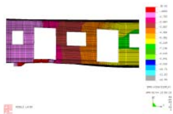
Fig. 2. Amount of deflection for vertical loading
