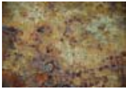
Fig. 12 Pitting corrosion of SS400 (corrosion for 3 months, \times 100 )
