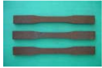
Fig. 6 Corrosion for 9 months(SM490A)
