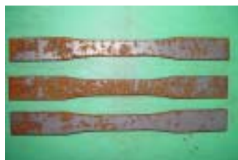
Fig. 2 Corrosion for 6 months(SS400)
