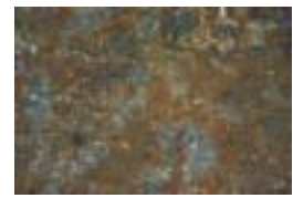
Fig. 15 Uniform corrosion of SM490A (corrosion for 6 months, \times 100 )
