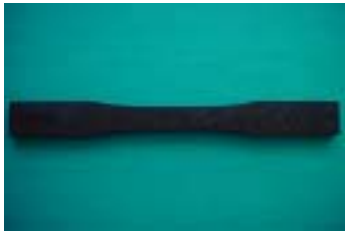
Fig. 4 Corrosion for 3 months(SM490A)
