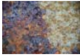
Fig. 13 Uniform corrosion of SM490A (corrosion for 3 months, \times 100 )
