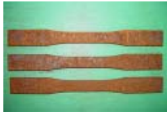
Fig. 5 Corrosion for 6 months(SM490A)
