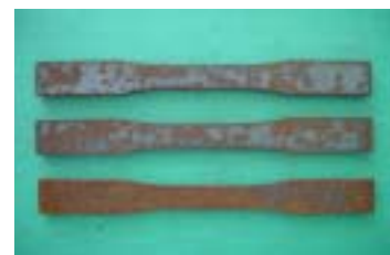
Fig. 3 Corrosion for 9 months(SS400)
