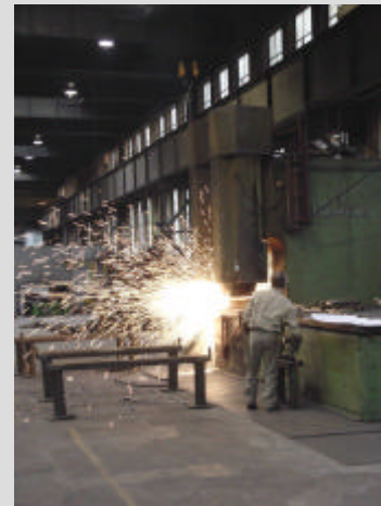
Welding the switch blade profile Fz36 to standard profile Ri 60 with transitional profiling
