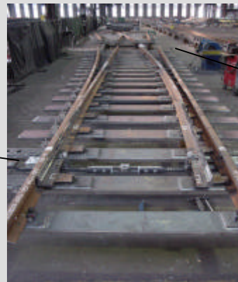
Switch for Railway
