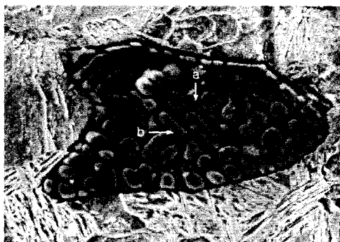
Fig. 6. SEM image of non-metallic inclusion of cross section (x1,000)
