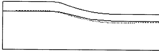
Fig.12 Cu-Al contact profile in an Eulerian mesh before and after correction using a stream line technique
