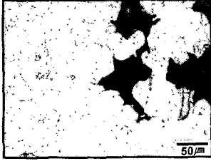
Fig. 4. Cavity formed around grain boundary
