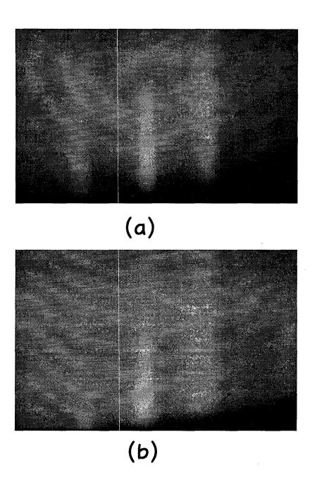
Fig 1. (a) RHEED pattern of GaSb 1000 Å on GaAs(100) substrate. (b) RHEED pattern of MnSb 1000 Å on GaSb buffer layer.
