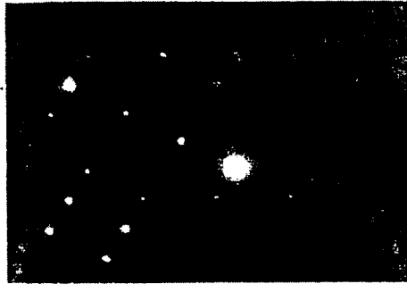
Fig. 3. Diffraction patterns of TEM for rod-shaped \gamma -LiAlO 2 particles using ammonium carbonate as a pore-former, which corresponds to a \gamma -LiAlO 2 single crystal.
