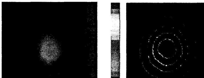
Fig. 2 Near-field pattern of a waveguide written inside fused silica glass using a 350 nJ, 1 kHz femtosecond laser pulses
