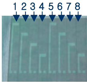
Fig. 6. Fabricated samples for measuring e_{31,f}
