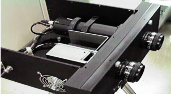
Fig.3 Phase-Shifting Projection Moire(Intek Plus, Co. Ltd.)
