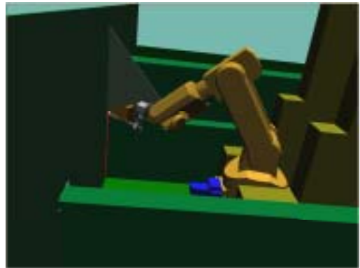
Fig. 9 Simulation of vertical welding
