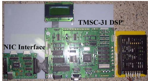
Fig. 8 TMS320C31 DSP and NIC interface board
