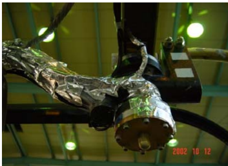
Fig. 8 Load cell under second suspension spring
