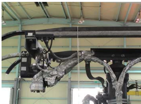
Fig. 7 Wire rope to connect pan-head with lift load cell
